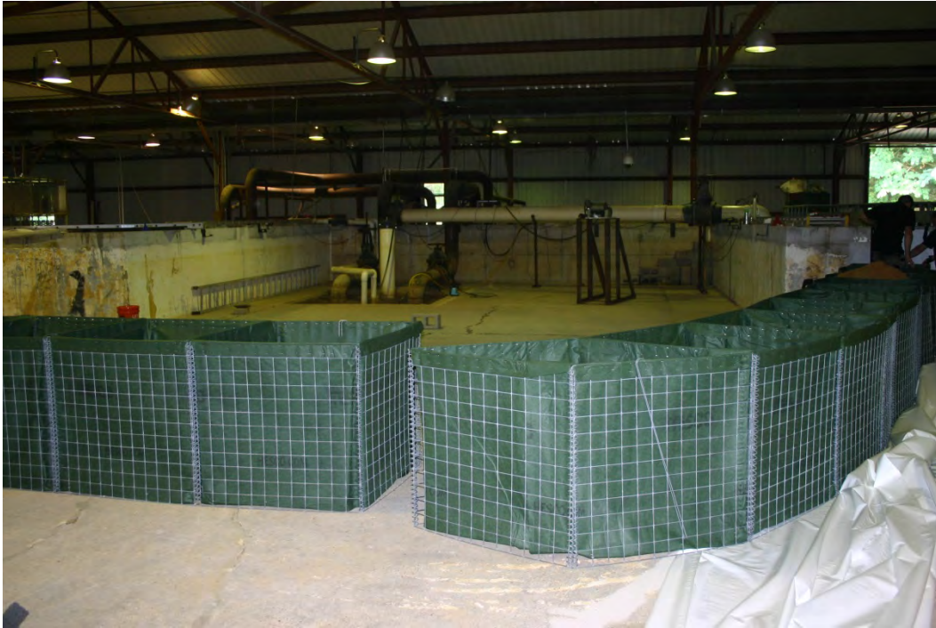
Figure 2. Looking into the test area of the research basin. The vertical white pipes extend down into the seepage pit. Barrier is not from actual test.
