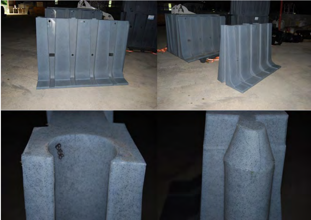
Figure 4. 4-Foot Muscle Wall barrier: front side (top left), perspective view (top right), female connector (bottom left) and male connector (bottom right).
