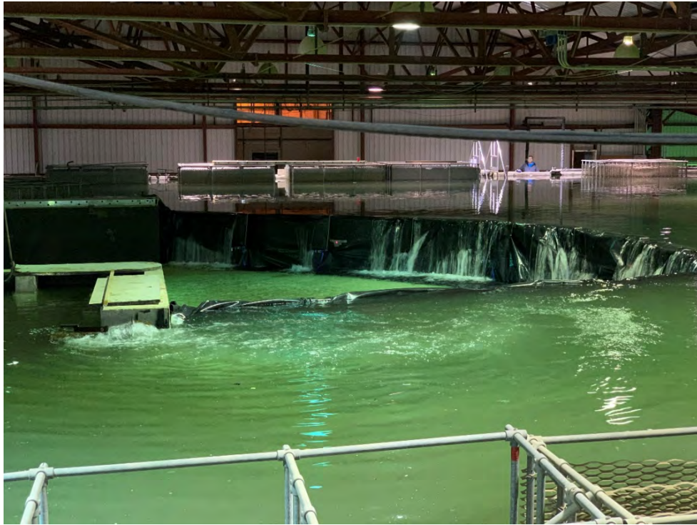
Figure 40. Overtopping of 4-Foot Muscle Wall during overtopping test.
