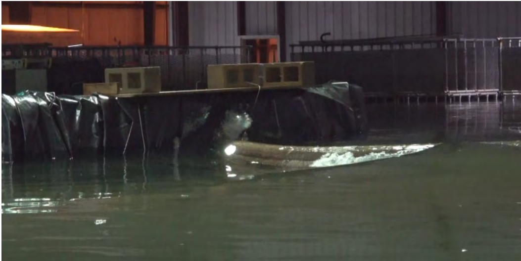
Figure 44. Snapshot of the large log impacting the center wall.
