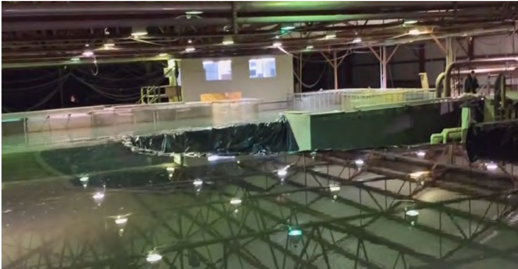
Figure 21. Barrier holding back water at 100 percent of structure height.
