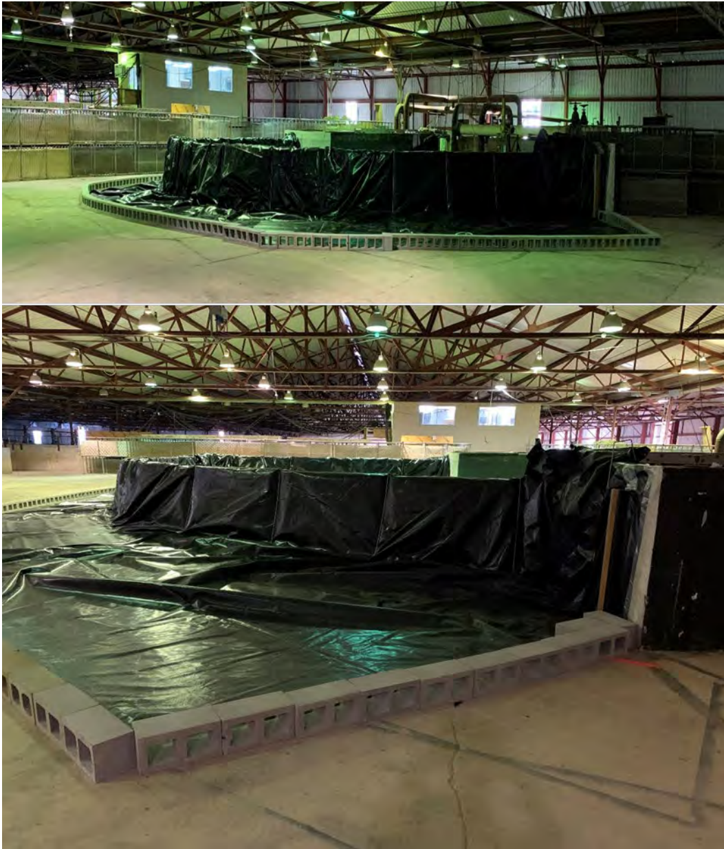
Figure 15. Front (top) and left (bottom) views of the assembled 4-Foot Muscle Wall flood barrier.
