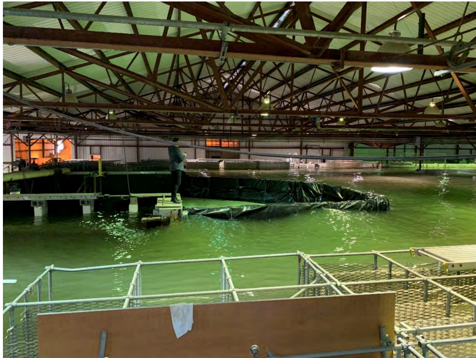
Figure 35. Flood barrier during the test with medium wave heights at high water.
