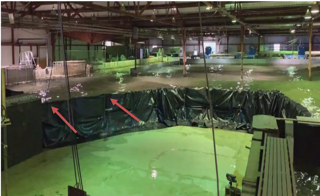
Figure 30. Overtopping during the test with large waves at low water.
